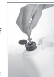
Figure 4: Open the bottle cap and press the Blue quick connect into the opening on the bottle.
